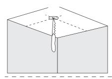
Cut opening in ceiling. See table for cutout dimensions. Cutout must be accurate and clean as oversized or jagged edges will prevent the luminaire from seating properly. A hole saw is recommended for a precise fit.
